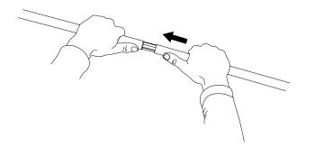
4. Should you pull out the tube too far, rectify this by removing it completely, taking off the wall bracket and pushing through from the other side.
